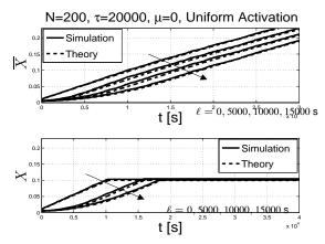
(a) Dynamics of the number of infected nodes under uniform activation, when  $\ell = 0,5000,10000,15000$ ; upper part (a.l) depicts uncontrolled dynamics, the lower one (a.ll) optimal dynamics for x = 0.1. Earlier the activation, more the infection and quicker the saturation.
