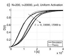
(c) CDF of the delay for optimal control : the thin solid lines represent the value attained by the uncontrolled dynamics. The case  $\ell = 0$  corresponds to plain Two hops routing.
